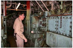
To give you another perspective of how large these diesels are, a single piston is about a foot in diameter and just over four feet long. For comparison, the piston in your car might be smaller than a can of frozen juice concentrate with a Popsicle stick sticking out of it. And remember that there are twelve of these pistons in each D-S diesel.
