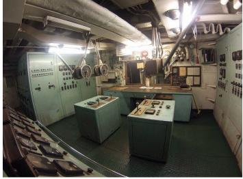
Notice in the picture above that the engine control room has four throttle controls on two pedestals nearly identical to those on the bridge. They were there "just in case". The Abby could be blindly powered ahead or astern from the engine control room while still being steered or helmed from up on the (navigation) bridge.
